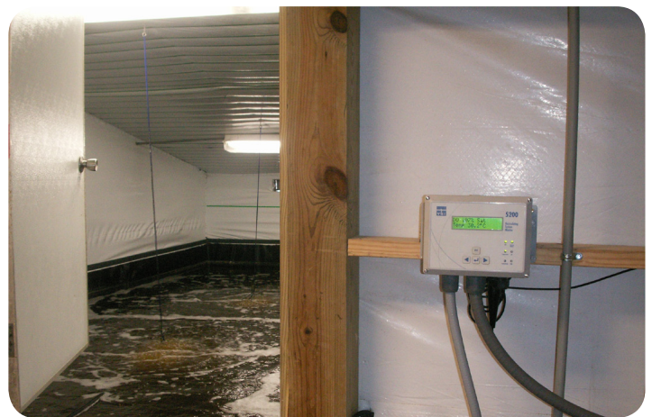
One of the NaturalShrimp tanks shown with the original YSI 5200 mounted outside
